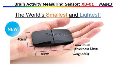
Attached on the back side of a hair band, the device measures and visualizes brain activity while the user is doing a quiz or game-like exercise on smartphone/iPad. The exercise program is customized for each user. The results are shown in real time on the smartphone/iPad. This enables the user to understand his/her own brain activity status and so provides an aid to improve daily life style.
