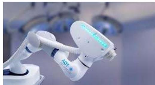
CARLO® allows surgeons to perform osteotomies with maximum precision and patient specific configurations based on CT (computer tomography) data. Surgeons have full control of the procedure while being assisted with a simple and intuitive 3D planning, navigation and control software and hardware which allow for preoperative planning but also intraoperative ad-hoc changes.
